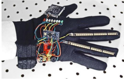
**Figura 2.9 - Exemplo luva com sensores extensômetro e giroscópio, retirada de [[http://grathio.com/2010/03/rock\\_paper\\_scissors\\_training\\_glove/](http://grathio.com/2010/03/rock_paper_scissors_training_glove/)].**
